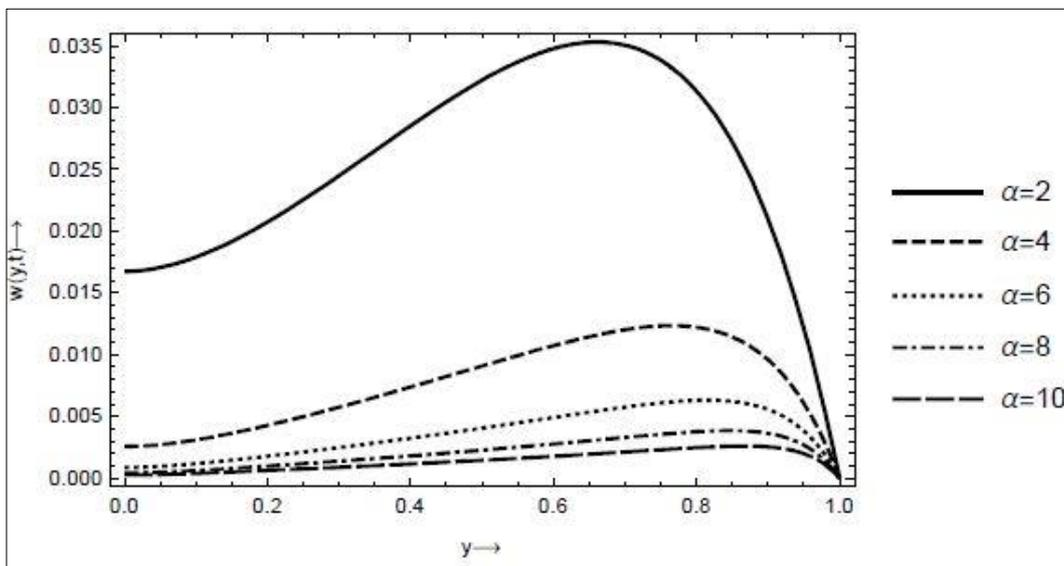
**Fig 5:** The effect of wave number on velocity profile, with  $Gr_t = 15, Nb = 1, Nt = 1, Sb = 2, Rd = 3, Re = 5, Gr_f = 15, Pr = 3, U_{hs} = 2, me = 2, a = 0.5, \epsilon = 0.4, \omega = 1, t = 5, P_0 = 0.05, x = 0.5$
