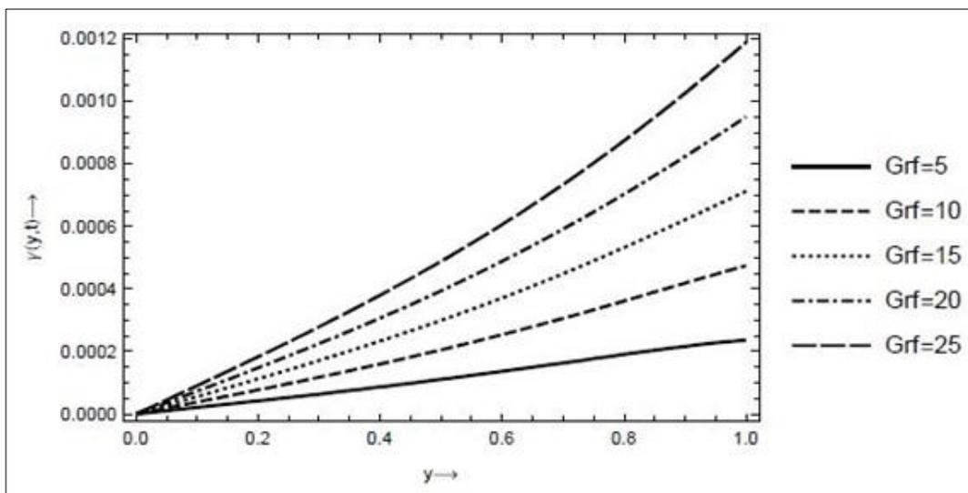
**Fig 7:** The effect of nanoparticles Grashof number on nanoparticles fraction profile, with  $Nb = 1, Nt = 1, Sb = 2, Rd = 2, \alpha = 3, Pr = 2.1, a = 2, \epsilon = 3, \omega = 2, t = 5, x = 0.5$
