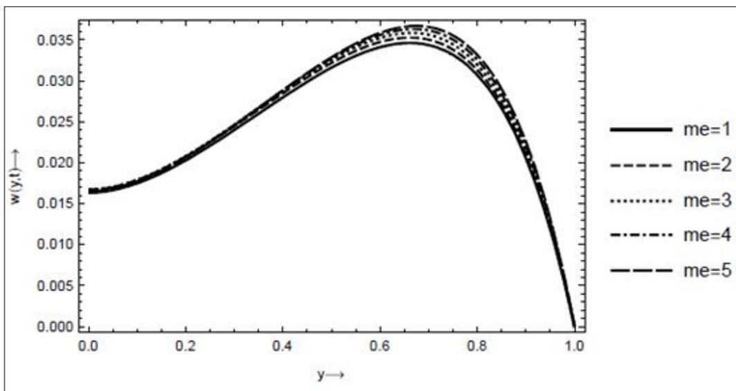
**Fig 6:** The effect of electroosmotic parameter on velocity profile, with  $Gr_t = 15, Nb = 1, Nt = 1, Sb = 2, Rd = 3, Re = 5, \alpha = 2, Pr = 3, U_{hs} = 2, Gr_f = 15, a = 0.5, \epsilon = 0.4, \omega = 1, t = 5, P_0 = 0.05, x = 0.5$
