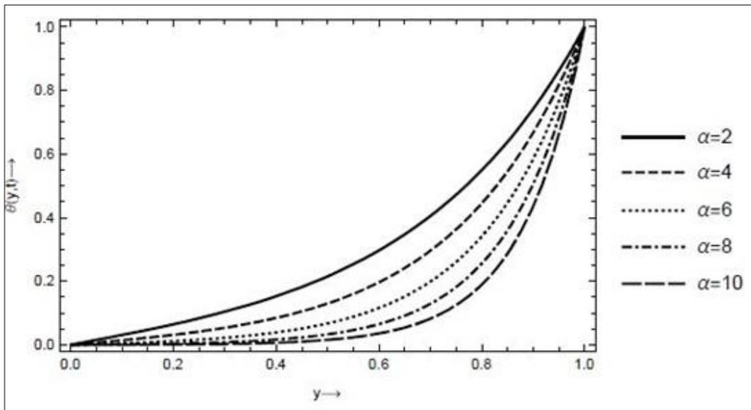
**Fig 11:** The effect of wave number on temperature profile, with  $Rd = 3, Pr = 2.1, a = 3, \varepsilon = 0.001, \omega = 0.3, t = 5, x = 0.5$
