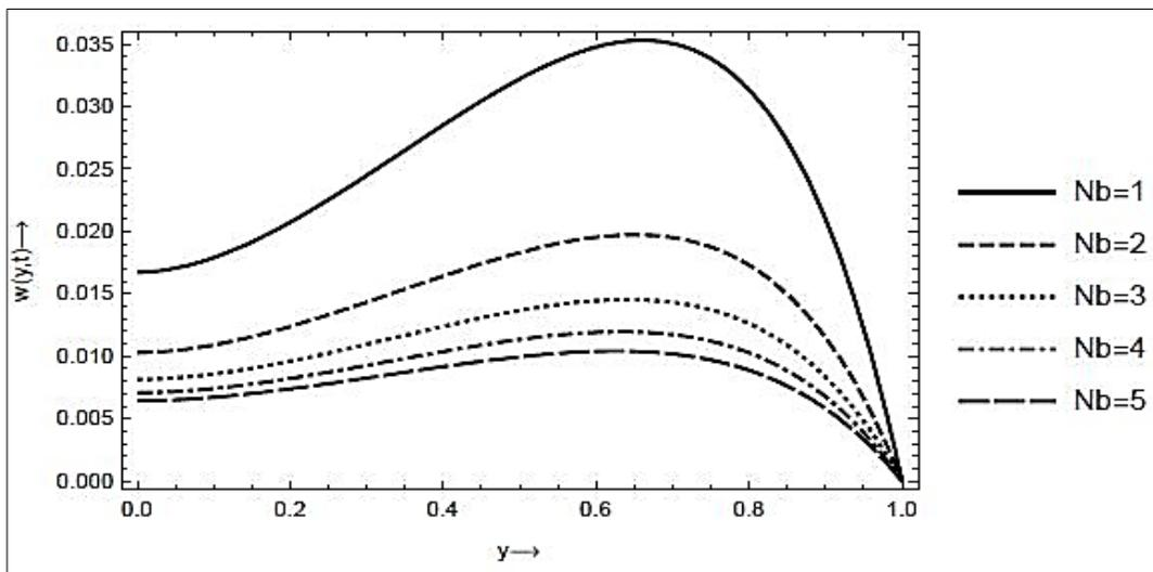
**Fig 3:** The effect of Brownian motion parameter on velocity profile, with  $Gr_t = 15, Gr_f = 15, Nt = 1, Sb = 2, Rd = 3, Re = 5, \alpha = 2, Pr = 3, U_{hs} = 2, me = 2, a = 0.5, \varepsilon = 0.4, \omega = 1, t = 5, P_0 = 0.05, x = 0.5$
