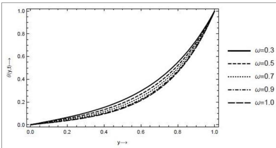
**Fig 12:** The effect of oscillatory parameter on temperature profile, with  $\alpha = 2, Pr = 2.1, a = 3, \varepsilon = 0.001, Rd = 3, t = 5, x = 0.5$
