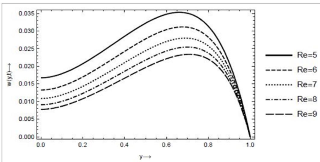
**Fig 4:** The effect of Reynolds number on velocity profile, with  $Gr_t = 15, Nb = 1, Nt = 1, Sb = 2, Rd = 3, Gr_f = 15, \alpha = 2, Pr = 3, U_{hs} = 2, me = 2, a = 0.5, \varepsilon = 0.4, \omega = 1, t = 5, P_0 = 0.05, x = 0.5$
