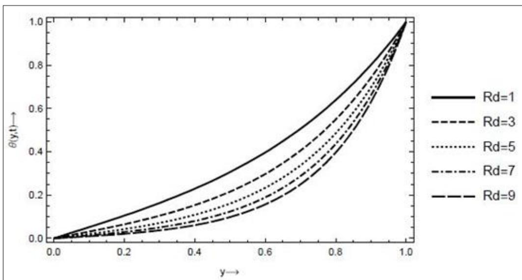
**Fig 10:** The effect of radiation absorption on temperature profile, with  $\alpha = 2, Pr = 2.1, a = 3, \varepsilon = 0.001, \omega = 0.3, t = 5, x = 0.5$
