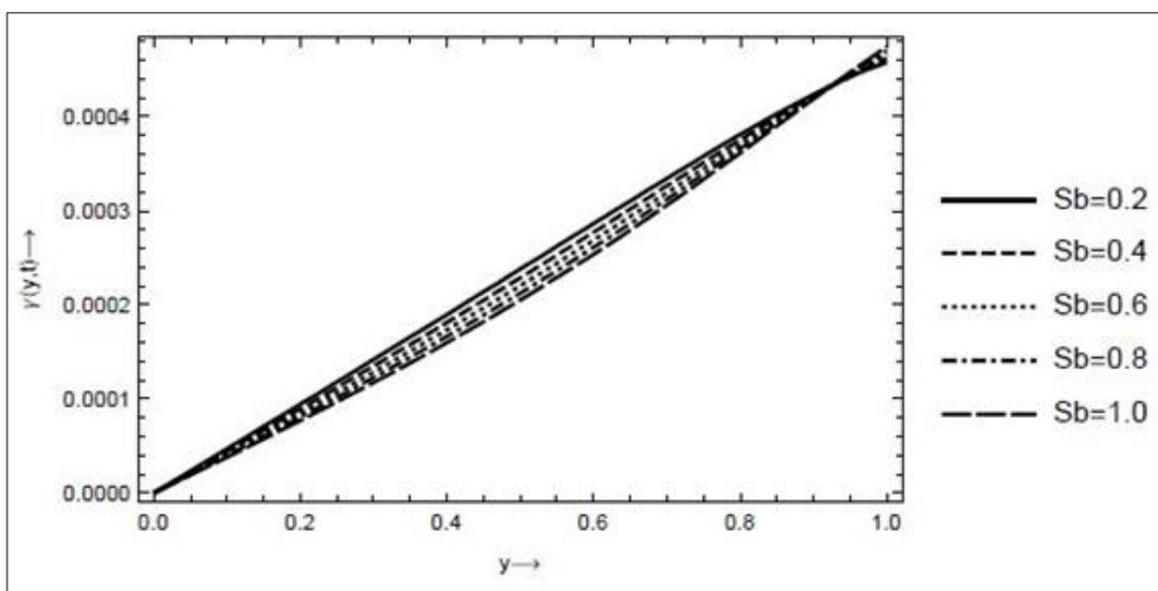
**Fig 9:** The effect of Schmidt number on nanoparticles fraction profile, with  $Nb = 1, Nt = 1, Sb = 2, Rd = 2, \alpha = 3, Pr = 2.1, a = 2, \varepsilon = 3, \omega = 2, t = 5, x = 0.5$
