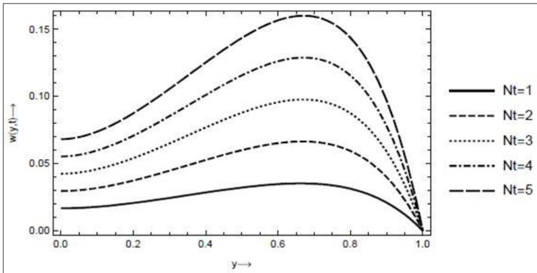
**Fig 2:** The effect of thermophoresis parameter on velocity profile, with  $Gr_t = 15, Nb = 1, Gr_f = 15, Sb = 2, Rd = 3, Re = 5, \alpha = 2, Pr = 3, U_{hs} = 2, me = 2, a = 0.5, \varepsilon = 0.4, \omega = 1, t = 5, P_0 = 0.05, x = 0.5$
