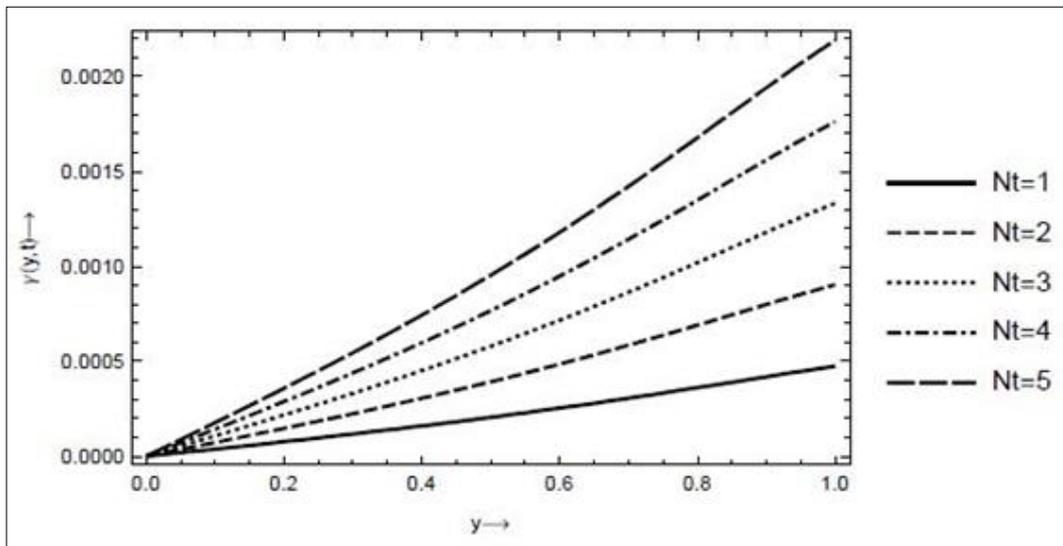
**Fig 8:** The effect of thermophoresis on nanoparticles fraction profile, with  $Nb = 1, Nt = 1, Sb = 2, Rd = 2, \alpha = 3, Pr = 2.1, a = 2, \varepsilon = 3, \omega = 2, t = 5, x = 0.5$
