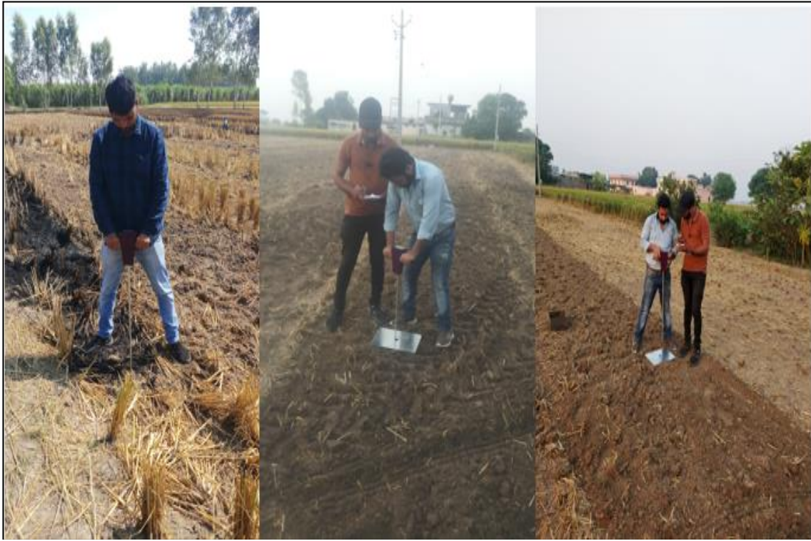
Fig 5: Soil profile recording with the Field SC 900 Cone Penetrometer
