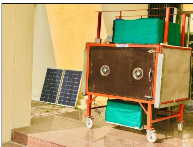
Fig 1: Developed portable solar assisted evaporative cool chamber
