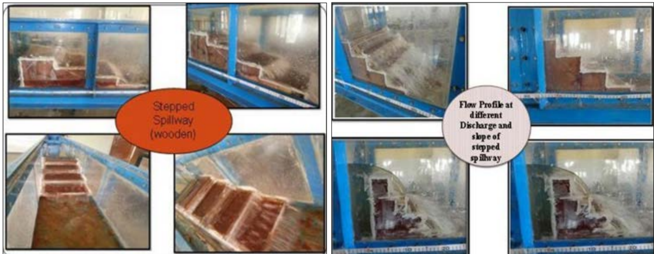
Fig 4: A Pictorial View of Stepped Spillway – Wooden, Showing Physical Configurations as well as flow patterns while placing it In Flume Channel
