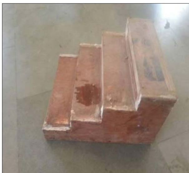
Fig 3: A Pictorial View of Stepped Spillway- Wooden, Showing Physical Configurations as well as flow patterns while placing it In Flume Channel
