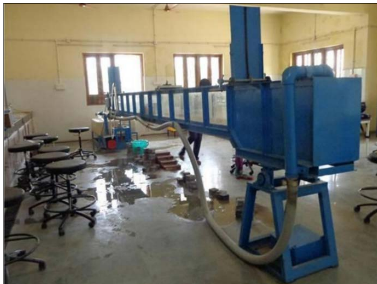
Fig 2: The real physical view of standard tilting hydraulic flume as adopted in present study
