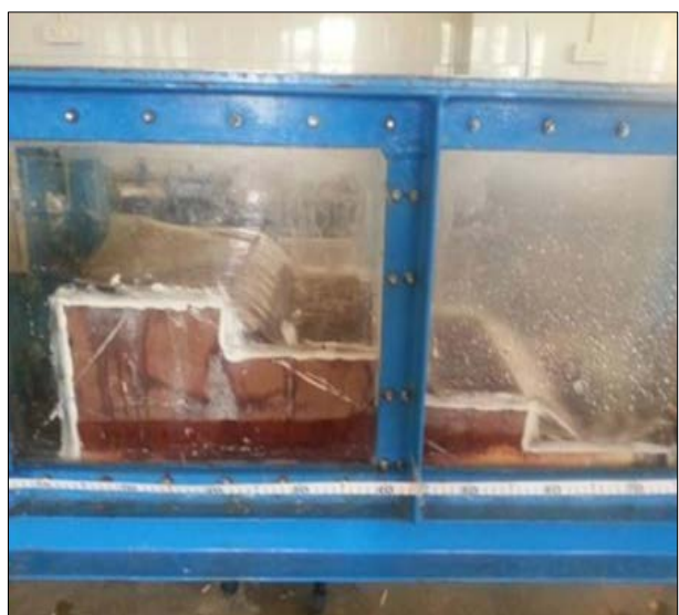
Fig 3: A Pictorial View of Stepped Spillway- Wooden, Showing Physical Configurations as well as flow patterns while placing it In Flume Channel
