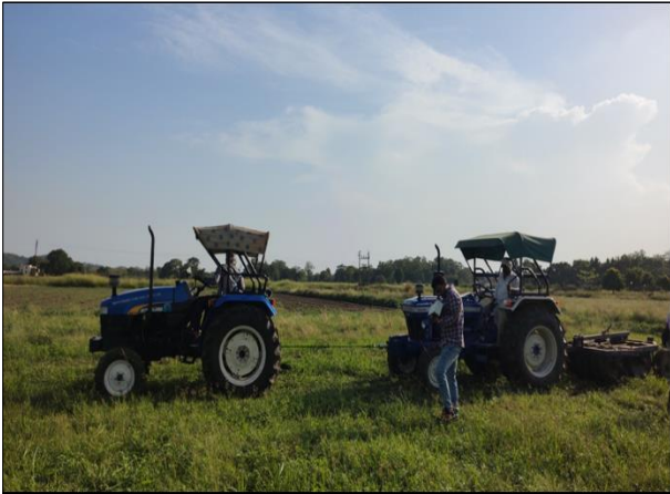
Plate 3: Draft force measurement (Dummy tractor method) by using tensile load cell
