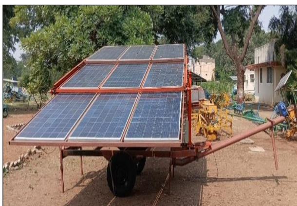
Fig 1: Solar power unit
