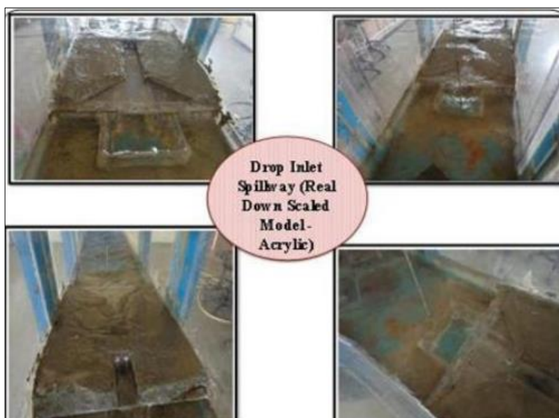
Fig 3: A Pictorial View of Down Scaled Drop Inlet Spillway with Straight Box Inlet-(Acrylic), Showing Physical Configurations as well as flow patterns while placing it In Flume Channel
