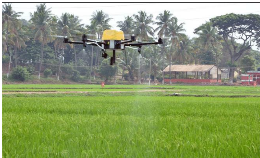
Fig 2: Hexa copter spraying pesticides in rice fields of Tamil Nadu Agricultural University Farm in Tamil Nadu, India during October 2019.
